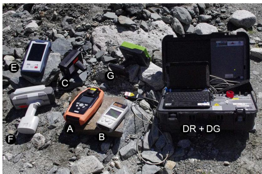
**Figure 2.** Miniature Raman spectrometers used in this study. FirstDefender XL (A), FirstDefender RM (B), Inspector Raman (C), EzRaman-I Dual using red laser (DR) and green laser (DG), Bravo (E), FirstGuard (F) and RaPort (G). [Colour figure can be viewed at [wileyonlinelibrary.com](http://wileyonlinelibrary.com)]
